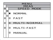
4-a-1. NORMAL or FAST setting: Select [NORMAL] or [FAST] and press ENTER key.
